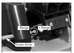
FIGURE 2 - ADJUSTING SENSOR RANGE Place the screwdriver through the access hole as shown to adjust sensor range. Range is set at the factory for 4 - 6 inches. Increase range to reduce air deflection noise.
