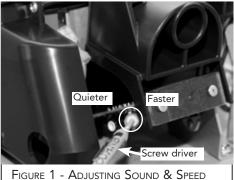
FIGURE 1 - ADJUSTING SOUND & SPEED The dryer is shipped set at maximum speed. Turn counterclockwise to reduce sound and speed 3/4 of a turn max.
